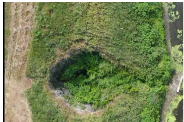
Picture #16: Severe Washout from Collapsed Tile in Section 18 of Sterling Township
