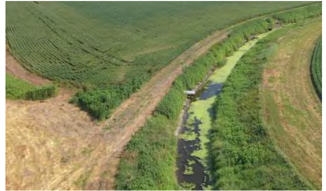
Picture #10: Unprotected Tile Outlet in Section 18 of Sterling Township.
