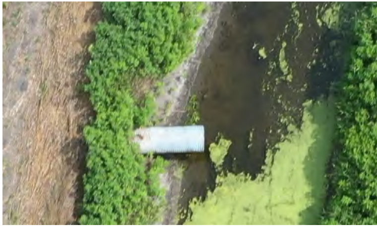
Figure 5. Unprotected Tile Draining into the Main Open Ditch
