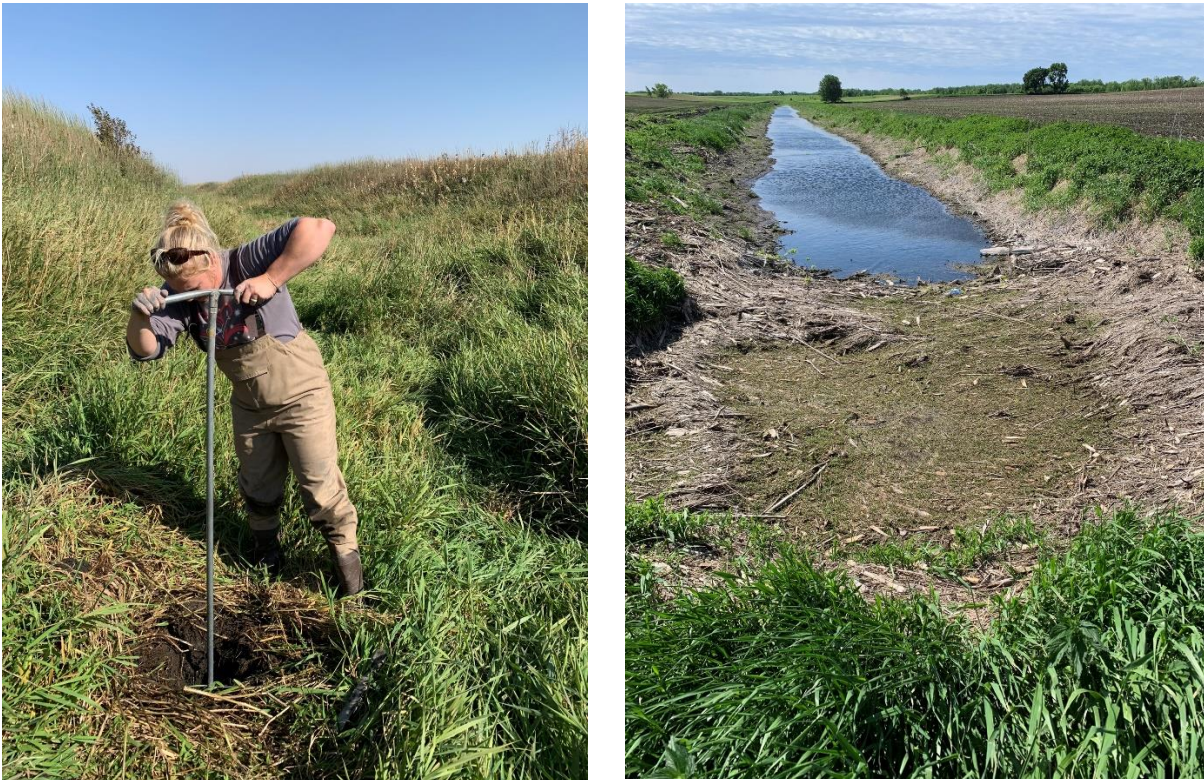
Figure 2. Left: Staff using a soil auger to locate the legal bottom of the open ditch. Right: Sediment accumulation in the open ditch.
