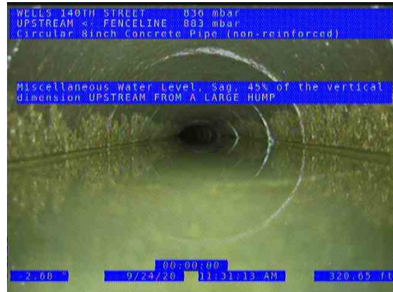
FENCELINE POINT (US) UPSTREAM_ccd425f4-2265-4a7f-b251-49792cea78a8_20200924_115332_828.jpg, 00:09:34, 320.65ft Miscellaneous Water Level, Sag, 45% of the vertical dimension / UPSTREAM FROM A LARGE HUMPS
