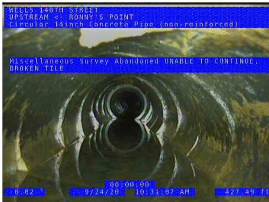
RONNY'S POINT (US) UPSTREAM_ec9d819f-136e-448f-b255-9ef79eb24f75_20200924_105325_883.jpg, 00:19:08, 427.49ft Miscellaneous Survey Abandoned / UNABLE TO CONTINUE, BROKEN TILE
