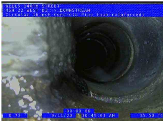
MSH 22 WEST DI (DS) DOWNSTREAM_5f0b4e20-2ff8-4939-833e-635333ce17e8_2 0200911_110927_927.jpg, 00:03:42, 35.50ft Tap Break-in Activity at 9 o'clock, dia/height: 6inch / CONCRETE
