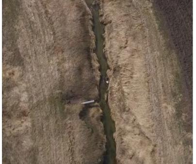
Figure 14: Unprotected Tile in the NE 1/4 of Section 12 Barber Township
