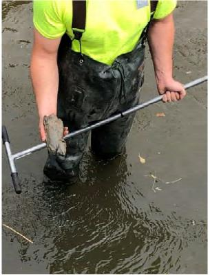
Figure 20: Soil Boring Sample showing Clay Layer
