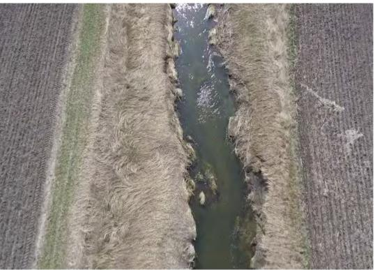
Figure 8: Sediment Buildup in NW 1/4 of Section 1 Barber Township
