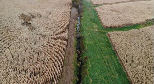
Figure 30: Steep Banks requiring Side Slope Flattening in Section 24 of Barber Township
