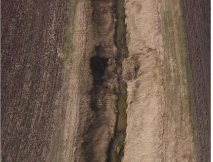
Figure 16: Sloughing Along Slope in the NE ¼ of Section 12 Barber Township
