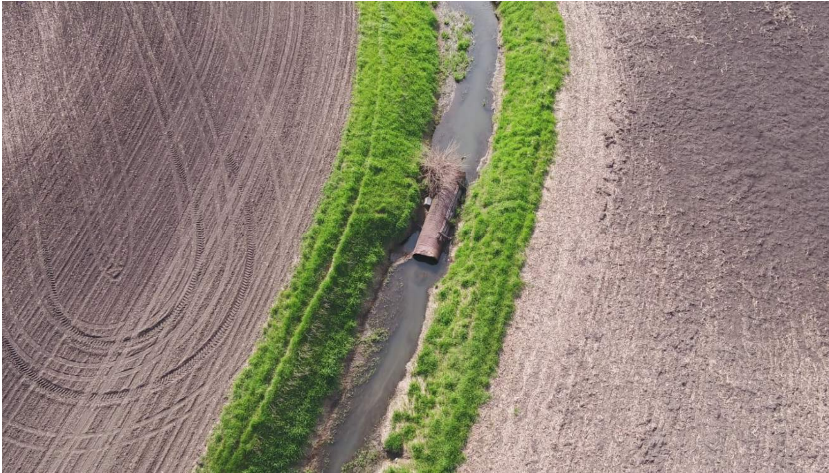
Drone Survey Photograph 4: Removed Field Crossing and Culvert Obstruction at Station 109+00
