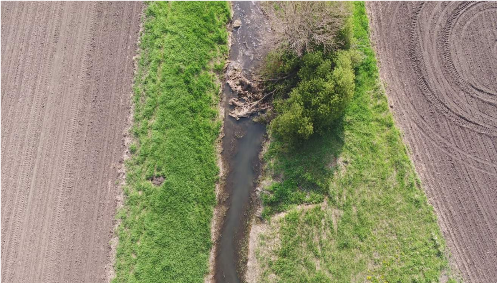
Drone Survey Photograph 5: Tree Obstruction at Station 121+00
