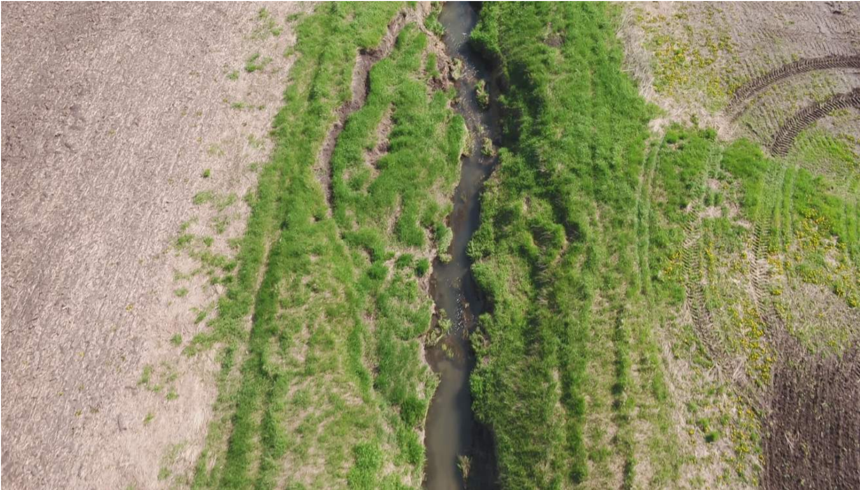
Drone Survey Photograph 2: Sloughed Bank at Station 14+00
