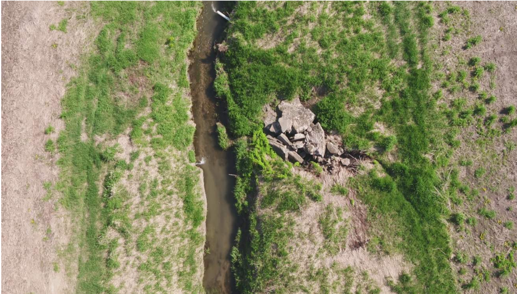
Drone Survey Photograph 1: Eroded Bank and Fill at Station 10+50
